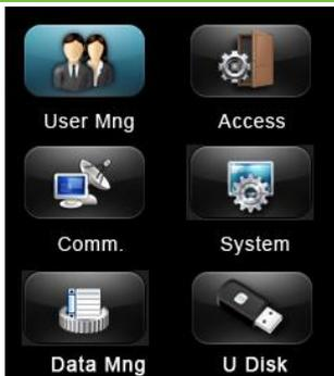
Press & hold **(MOK)** key to enter the **Main menu** interface; include **User Management (User Mng)**, **Access Setting (Access)**, **Communication Setting (Comm.)**, **System Setting (System)**, **Data Management (Data Mng)** and **U Disk Management (U Disk)**.
