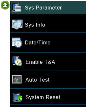
**Sys Parameter:** Set **Threshold (1:1)**, **Match Threshold (1:N)**, **Date Format**, **Sleep time**, whether enable **Key tones/Voice** and adjust **Volume** as required.
