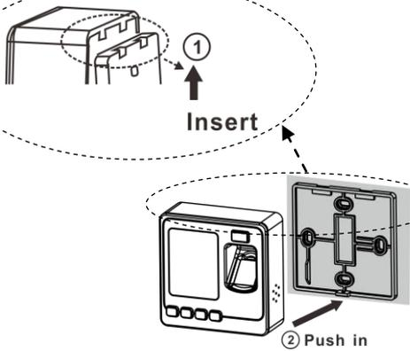
4. Fix the device on the Back Cover.
