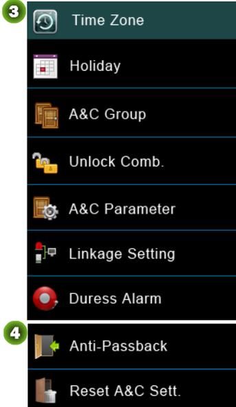
**Time Zone:** Add **Time Zones** for device. The device controls access according to the Time Zones.
