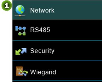
**Network:** Set IP address (The default value is 192.168.1.201), **Subnet mask** (The default value is 255.255.255.0) and **Gate Way** (The default value is 192.168.1.254) for device.
