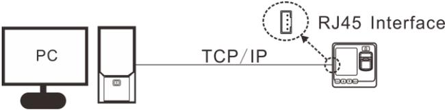
Connect with PC through TCP/IP network
