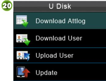
**Download Attlog:** Download all attendance logs to the U Disk. And then import logs into the **Access 3.5** software through **Import Data From USB disk** function, and then view Access Report as required.
