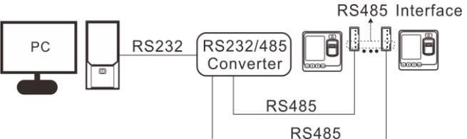
The diagram of system construction
